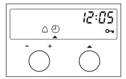
Use the **A Function dial**, for selecting oven functions which require input e.g. the time of day.
